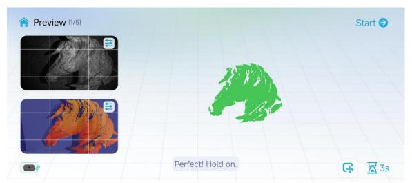
The preview phase mainly provides RGB images/depth images, IR images, and real-time point clouds for preview, alignment, and judgment of the current point cloud quality. The RGB/depth preview window and IR preview window provide nine squares for alignment of the scanner's field of view. It is recommended to keep the scanning portion in the center area of the preview window.
