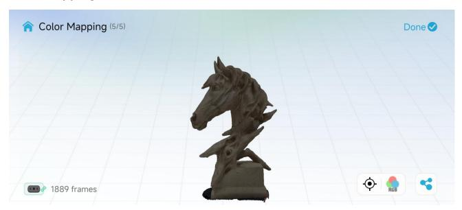
The last step of the scanning process is the generation and display of the mapped model.
